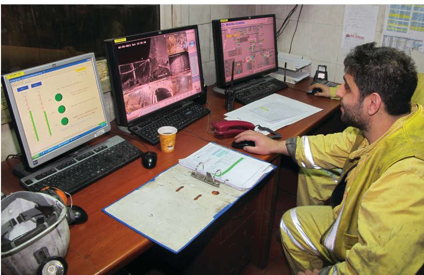
Figure 4. Backfill plant operator monitoring barricade pressures and video feed in real time, in order to optimize slope filling.
